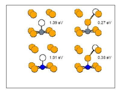
Figure 2. Binding energies between C (top) and N (bottom) impurity and vacancy positioned in 1NN and 4NN in bcc-W
